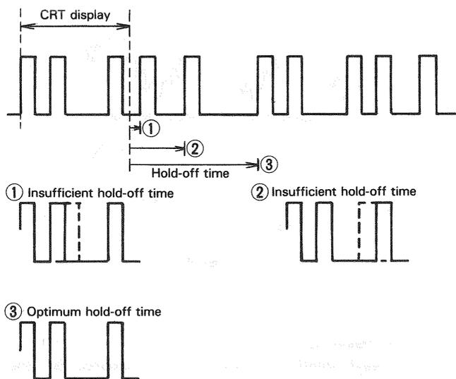
5. Adjust the SWEEP TIME/DIV control (26) to obtain an appropriate display. Now a normal sweep display is obtained.
