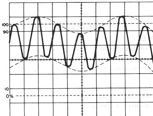
Signal containing undesired component
