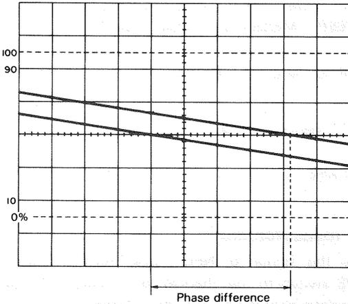
Expanded sweep waveform display.
